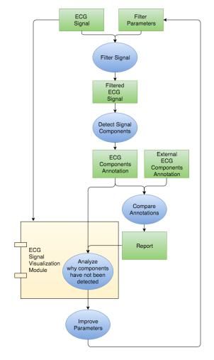
Fig. 3. An iterative process on how the ECG signal visualization improves the overall effectiveness
