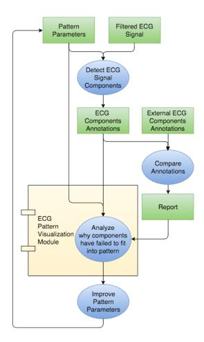
Fig. 4. An iterative process on how the pattern visualization model improves the overall effectiveness
